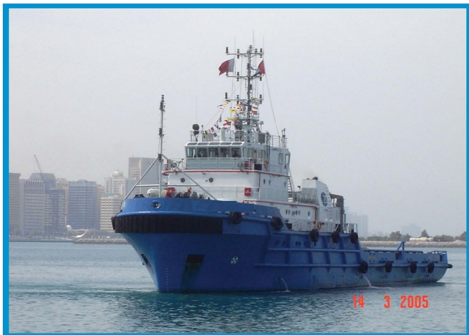
59.9M 4000 BHP ANCHOR HANDLING TUG SUPPLY VESSEL
